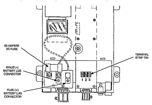
FIGURE 2. BATTERY CHARGER WIRING CONNECTIONS
